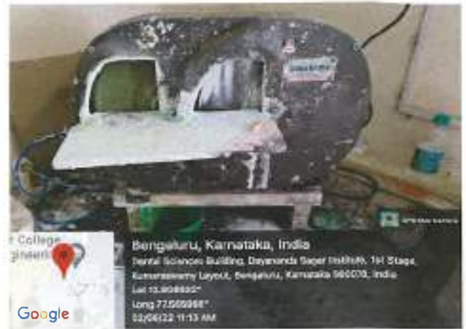
Double Disc Model Trimmer – to trim gypsum models and casts
